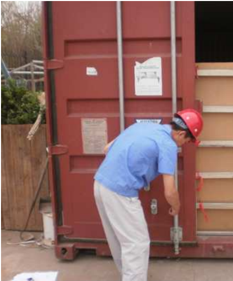
15. Fix the smaller warning tag on the second metal bar.
