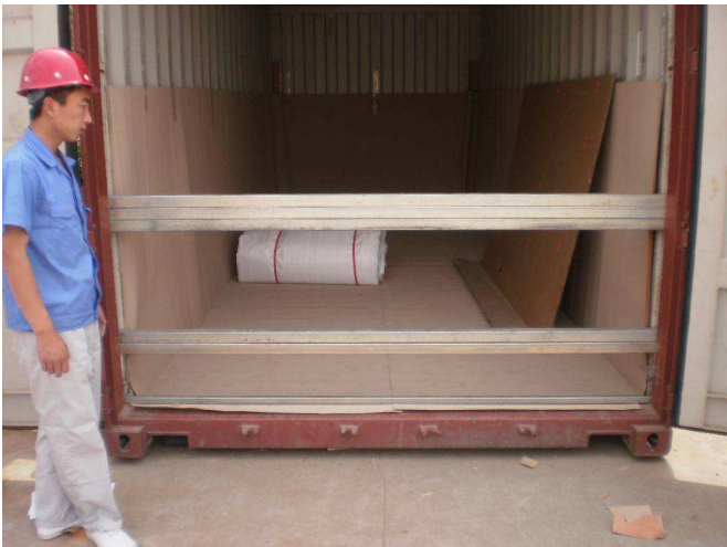
11. One installing staff goes inside of container and press the cardboard bulkhead against metal bars.
