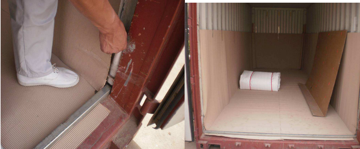
9. Crush another PVC tube at one end and insert it into the container corner
